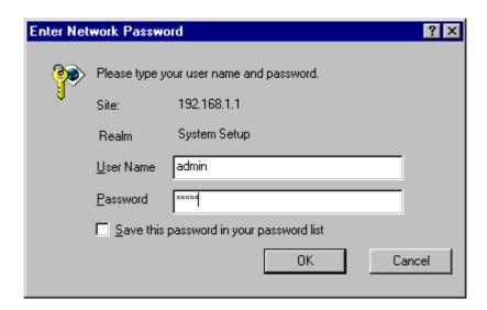
3. Enter the password to login onto the Wireless Access Point. Both the default id and password are admin. The main page will show up.
